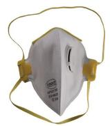
Respirator with valve, filter media in melt-blown electrostatic polypropylene, outer and inner layers in polypropylene SMS, twin strap from natural rubber, nose clip, foam nose cushion.
